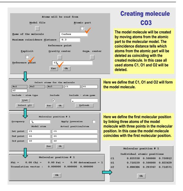
After creating the CO<sub>3</sub> molecule the header of M40 changes as shown in the next scheme. The molecular part of M40 starts with name *Carbox* of the model molecule followed by name of the reference point and by atoms of the model. Then the first position pos#I follows. It has zero rotations and translations because the atoms of the model molecule are already in the position.
