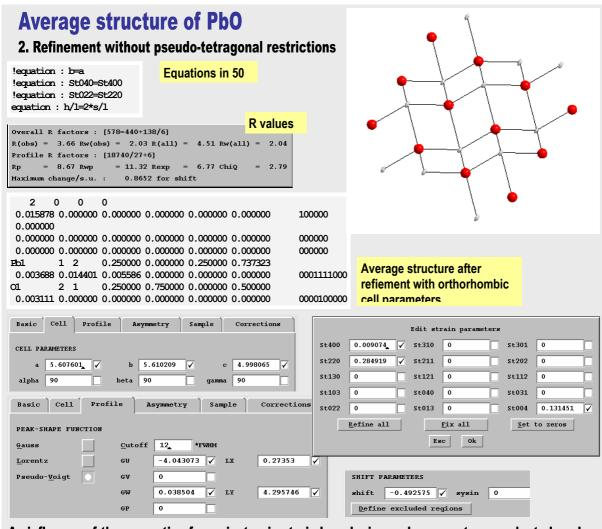
An influence of the correction for anisotropic strain broadening and asymmetry on selected peaks.
