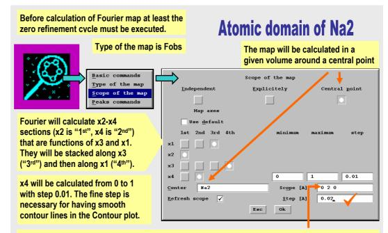
The map will be calculated for x1, x2, x3 in intervals corresponding to the volume  $<x1_c-0,x1_c+0>,<x2_c-1Å,x2_c+1Å>,<x3_c-0,x3_c+0>$  around the central point  $(x1_c,x2_c,x3_c)$  = position of Na2 in the basic structure, with step of 0.1Å.
