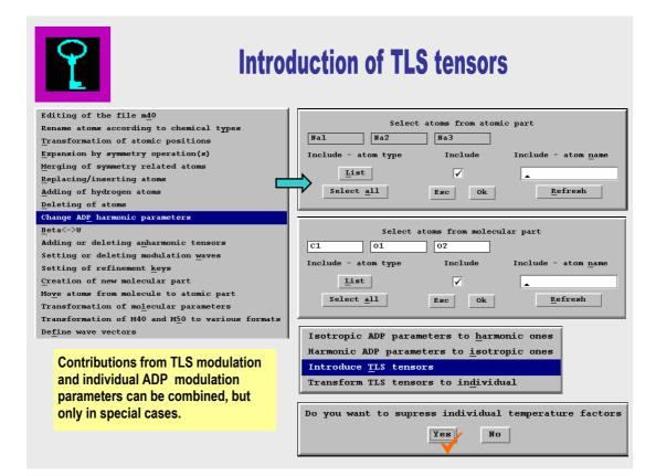
In M40, there are now no individual ADP in the model molecule. Amidst the molecular parameters of pos#1 there are new 21 parameters, six for the tensor *T*, six for *L* and nine for *S*. In fact, there is no saving of parameters by introducing TLS, as our CO<sub>3</sub> group is too small.
